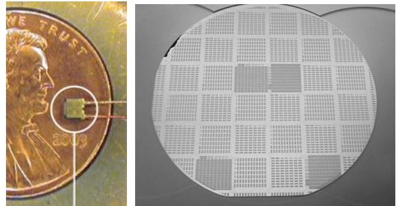
**Figure 7: Nextreme (left) thin-film TE cooler and MicroPelt (right)  $\text{Bi}_2\text{Te}_3$  thin-film TE wafer.**
