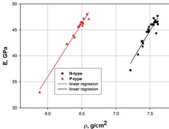
**Figure 2:** Variation of Young's modulus as a function of sample density for the N- and P-type rods.
