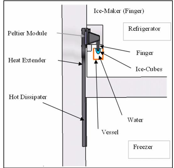
Fig. 4: Scheme of the system to model.
