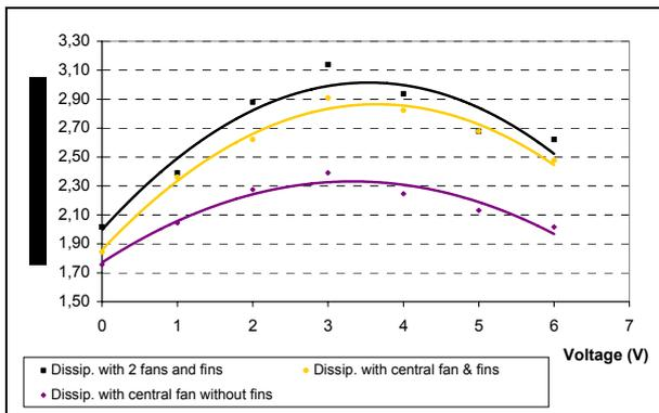
Fig. 7. Production of ice per day as a function of the voltage of the Peltier module.
