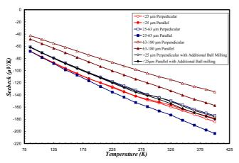
Figure 6: Temperature dependence of Seebeck coefficient of  $K_2Bi_8Se_7S_6$  pellets constructed with various particle sizes and measured parallel and perpendicular to pressing direction
