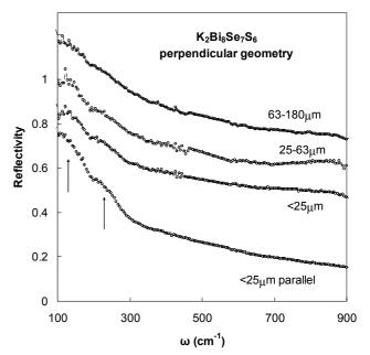
Figure 5: IR reflectivity spectra of K<sub>2</sub>Bi<sub>8</sub>Se<sub>7</sub>S<sub>6</sub>for different samples at various grain sizes. Spectra are shifted vertically for clarity
