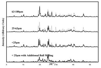
Figure 4: Powder X-ray diffraction pattern of  $K_2Bi_8Se_{13-x}S_x$ (x=6) pressed pellets parallel and perpendicular to the pressing direction.
