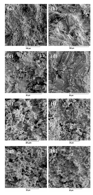
Figure 3: The SEM microstructure of sintered pellets parallel (a,c,e, g) and perpendicular(b,d,f,h) to the pressing direction. Pellets are fabricated with various grains size, (a,b) 63-180 $\mu$ m, (c,d) 25-63 $\mu$ m, (e,f) <25 $\mu$ m and (g,h)<25 $\mu$ m with5min additional ball milling.
