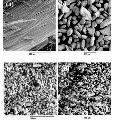
Figure 2: SEM images of  $K_2Bi_8Se_{13-x}S_x$  (x=6) (a) needles (cleaved ingot), powder after ball milling and sieving process (b)63-180µm, (c)<25µm and (d)<25µm with additional ball milling.
