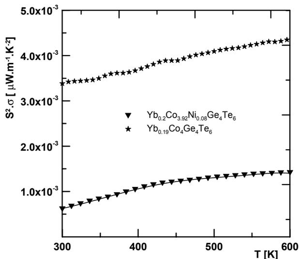
Fig.6: The comparison of power factors for  $\text{Yb}_{0.2}\text{Co}_{3.92}\text{Ni}_{0.08}\text{Ge}_6\text{Te}_6$  and  $\text{Yb}_{0.19}\text{Co}_4\text{Sb}_{12}$  [15].
