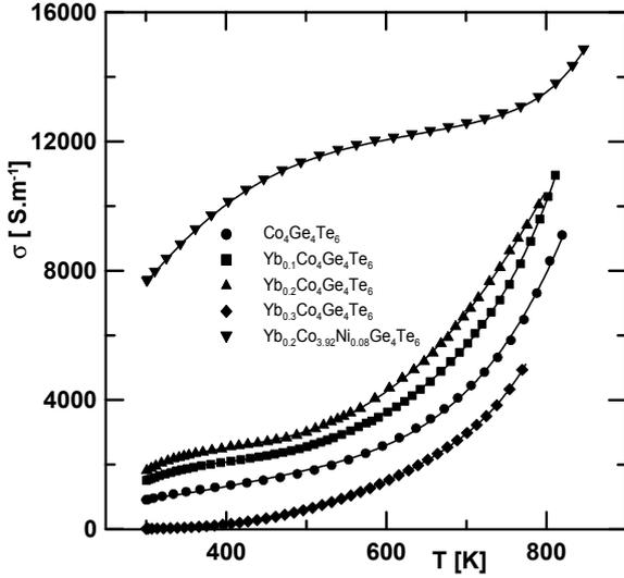
Fig.3: Electrical conductivity of the studied samples vs. temperature from 200 to 800 K.
