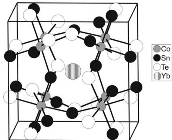
Fig.1: The representation of the structure of the skutterudite-related phase  $\text{Yb}_x\text{CoGe}_{1.5}\text{Te}_{1.5}$ ,  $R\bar{3}$  (rhombohedral setting).
