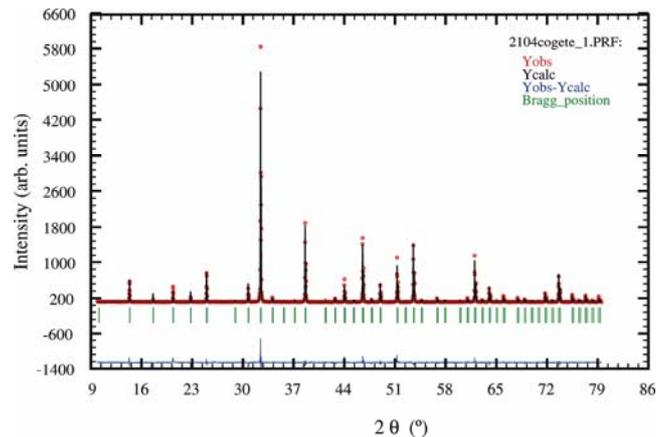
Fig.2: Observed (dots), calculated (solid line) and difference Rietveld profiles (the lowest line) for  $\text{Co}_4\text{Ge}_6\text{Te}_6$ . The vertical bars indicate the positions of Bragg reflections.
