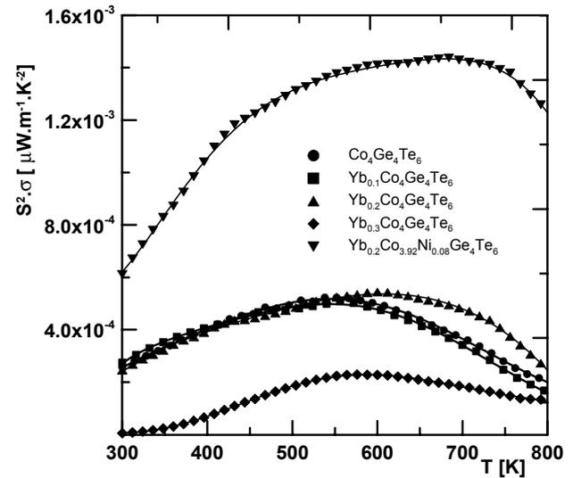
Fig. 5: Temperature dependence of power factor  $S^2\sigma$  of the studied samples
