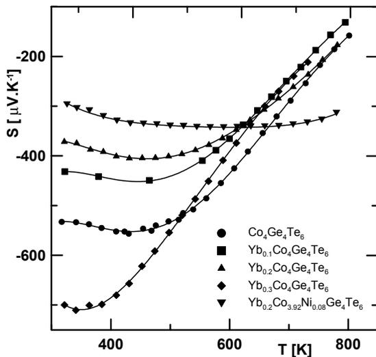
Fig. 4: Seebeck coefficient of the studied samples vs. temperature from 200 to 800 K.
