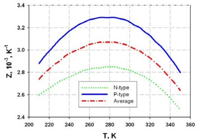
**Figure 1:** Variation of the thermoelectric figure of merit as a function of temperature for the N- and P-type rods.
