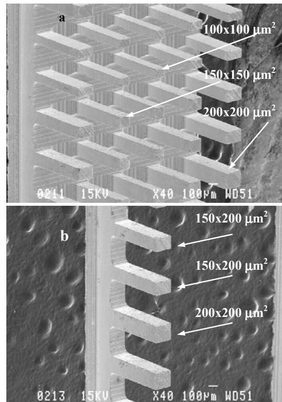
**Figure 6:** Scanning electron microscope images of N-type (a) and P-type (b) 1 mm thick wafers of extruded alloys after test cutting with a diamond blade.
