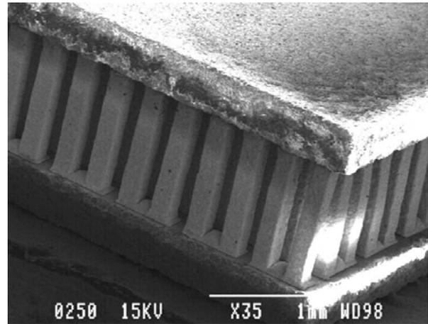
**Figure 5:** Scanning electron microscope observation of the micro module produced by Thermix Ltd (Ukraine) with legs 1.27 mm long and square sections of  $210 \times 210 \mu\text{m}^2$  cut by EDM.
