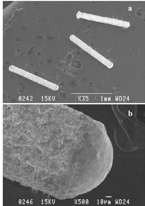
**Figure 3:** Scanning electron microscope observation of the legs with square sections of  $150 \times 150 \mu\text{m}^2$  cut by EDM from the N- and P-type rods (a) and leg end with Ni coating and soldering alloy wetting (b).
