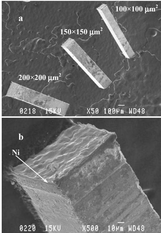
**Figure 4:** Scanning electron microscope observation of the 1 mm long legs with different square sections cut by diamond blade from the N-type Ni plated wafer (a) and  $100 \times 100 \mu\text{m}^2$  leg end with Ni coating (b).
