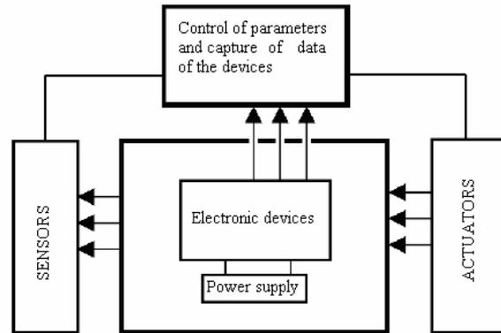
fig.3 Functional Description of the electronics
