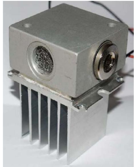
fig.6 Humidity actuator system including polymer.
