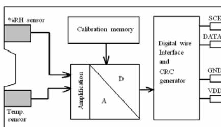
fig.5 Temperature and humidity sensor.
