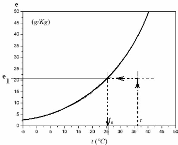
fig.2 Specific humidity vs. temperature
