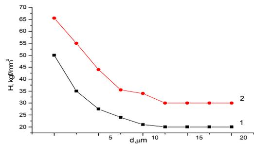
Fig. 3. The dependence of the microhardness on the microwire diameter.
