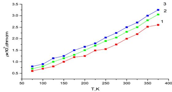
Fig. 8. The temperature dependence of the resistivity of the samples of type p treated at the temperature 450 K in the time interval: 1 - 1 hour, 2 - 72 hours, 3
