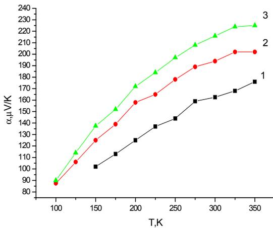
Fig.5. The temperature dependence of the thermopower of the samples of type p: 1 – before annealing, 2 - after annealing at the temperature 473 K, 3 - at the temperature 520 K. Time of annealing is 24 hours.
