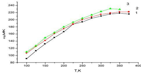
Fig.7. The temperature dependence of the thermopower of the samples of type p treated at the temperature 450 K in the time interval: 1 - 48 hours, 2 - 96 hours, 3 - 72 hours.
