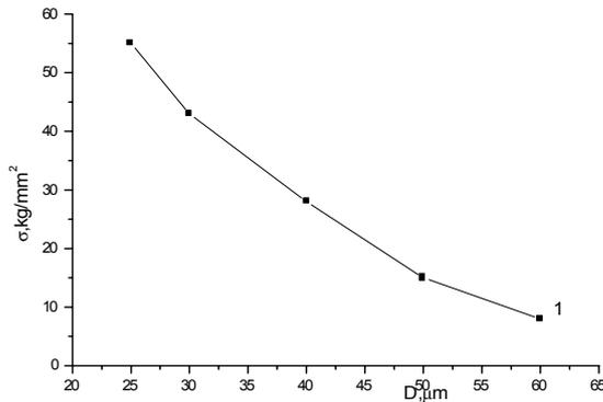
Fig.4. The dependence of the microwire durability on the cover diameter for nontreated samples (1) and the ones treated by annealing (2).
