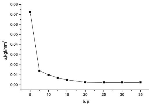
Fig. 2. The dependence of the wire tension on the diameter.
